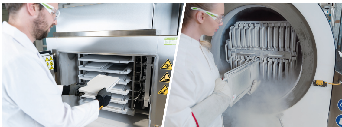
Controlled-rate freezing of small single-use bags with Single Use Support's plate freezer and LN2 freezer
